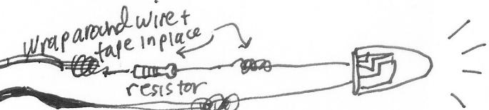
tape a pipe cleaner around the LED & wires so it can also be maneuverable. Sometimes the light source should be from below (glass slides) sometimes from above (rocks, etc.) but tape where you need it at the moment.
